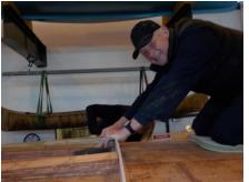
In the photo over left that is the hand of Harry using a shaped gauging batten to set up some of the internal transverse webs which will run between the internal intermediate step longitudinals.. Over left middle photo lan P is locating one of the step patterns
