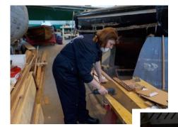
Seb, Below middle Tracie B is cleaning up a very rusty old cross cut saw that is due to be used in the shipwright's demos, Fay made up a new handle and Fred Sharpened it. Below
