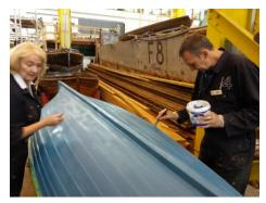
Over left Susan D and Linden T are giving the hull another undercoat and above right John S has just given the hull a light rub down with some very fine
